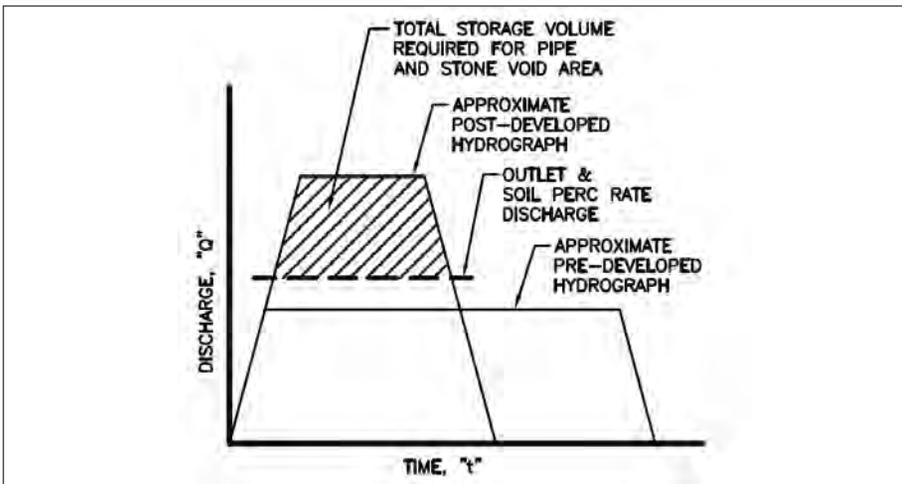
■ **Figure 6.3** Post-developed vs. pre-developed hydrograph retention with outlet.
