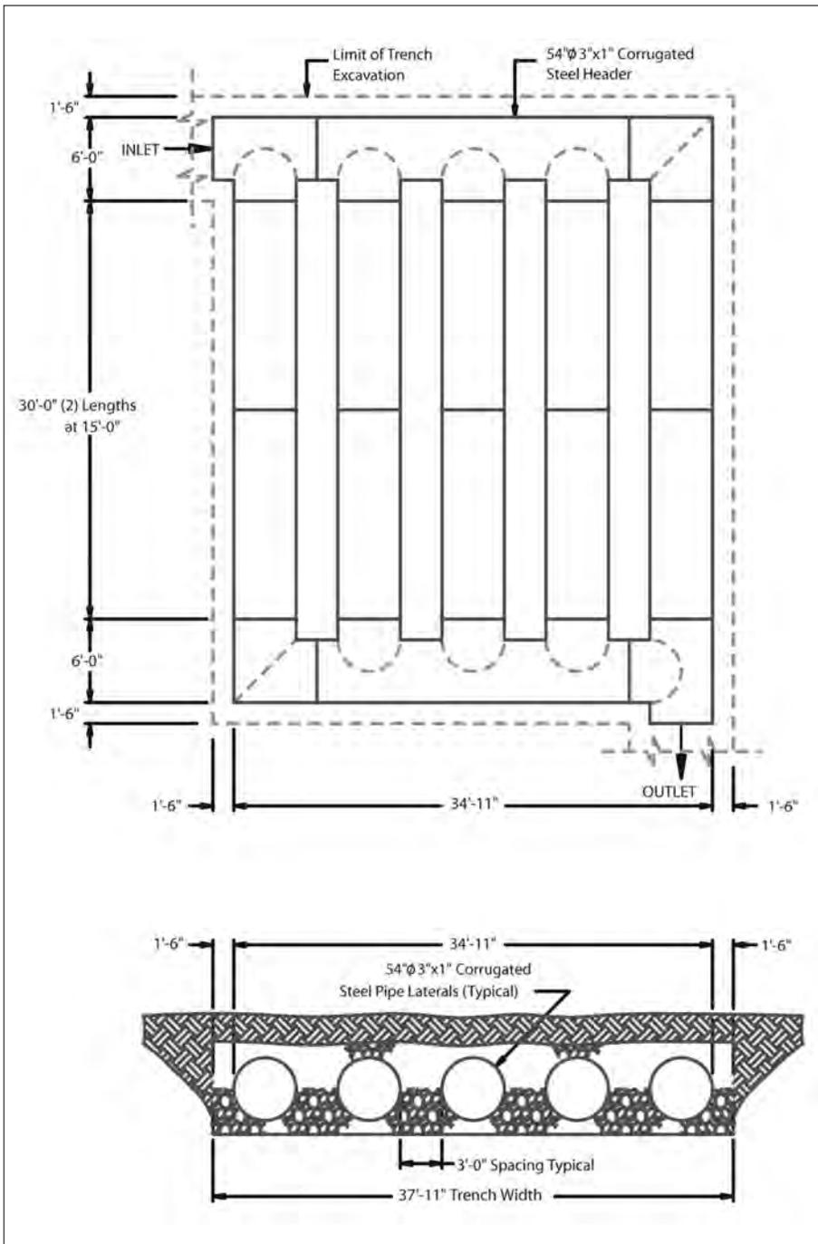
■ **Figure 6.6** Detention system layout for design example.
