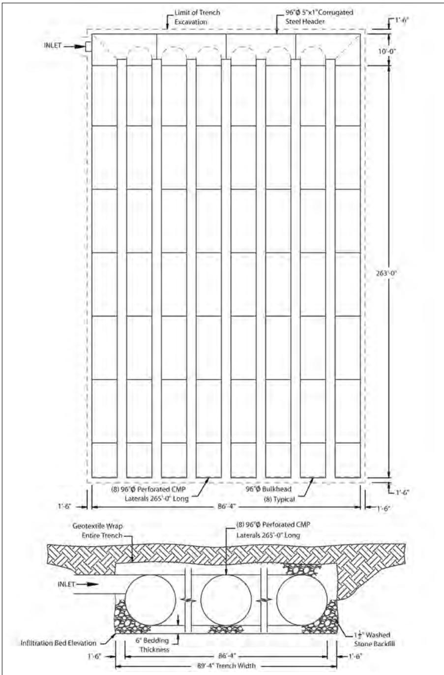
■ **Figure 6.7** Retention system layout for design example.
