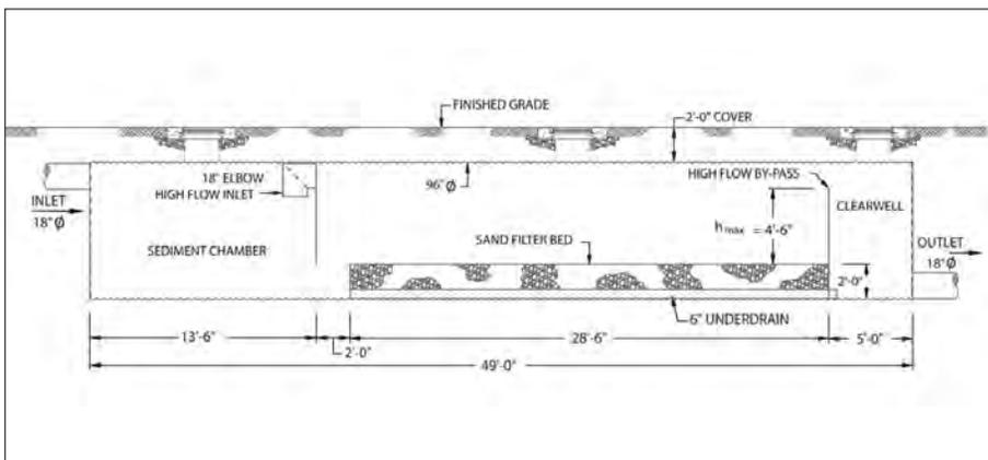
■ **Figure 6.9** Sand filter layout for design example.
