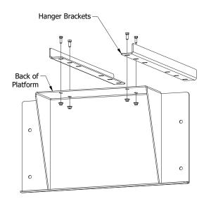
1. Attach 2 hanger brackets to back of reel platform with 4 bolts and nuts through the first 2 holes of hanger brackets (legs of hanger brackets must be oriented outward as shown)
