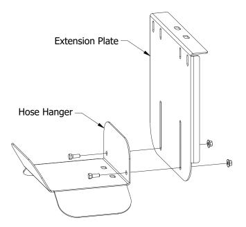
1. Assemble hose hanger and extension plate with two 3/8" bolts and nuts
