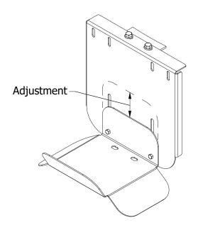
4. Loosen 3/8" bolts to adjust up or down to desired elevation and re-tighten
