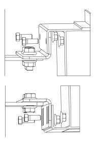
5. Secure reel to upper and lower brackets with four 3/8" bolts and nuts
