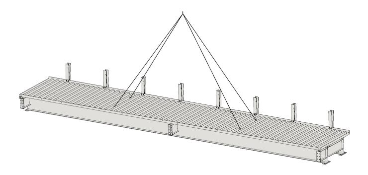
If bridge decking has not been pre-installed, bridge sections may be lifted utilizing four lift points at 1/4 to 1/3 span points as measured from the ends of the bridge section.
