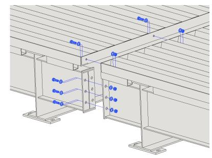
are to be installed tight. The fixed end of the bridge will have one bolt tighten according to the chart below. Expansion end will have two nuts per bolt. The first nut tightened finger tight to the washer placed on the bearing plate. The second nut will be installed tight to the first.
