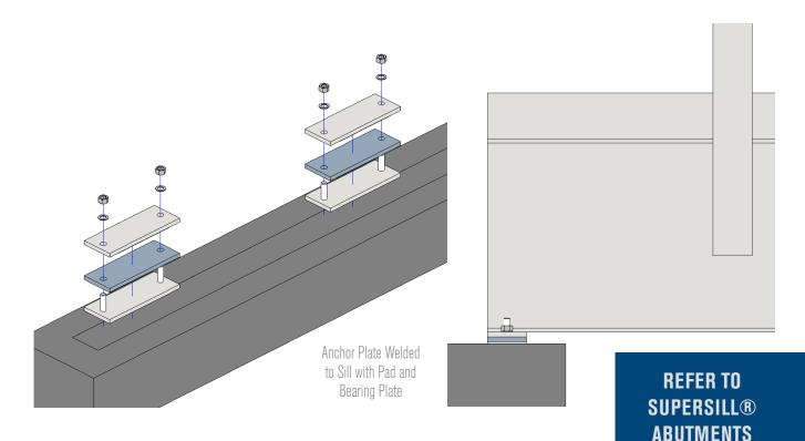
All bearing plates must be at the correct elevation, and ensure that there is uniform bearing between the abutment and leveling pad. If necessary, shim the plate with steel shims or use non-shrink grout under the entire bearing pad assembly in order to assure uniform bearing and the specified final elevation.
