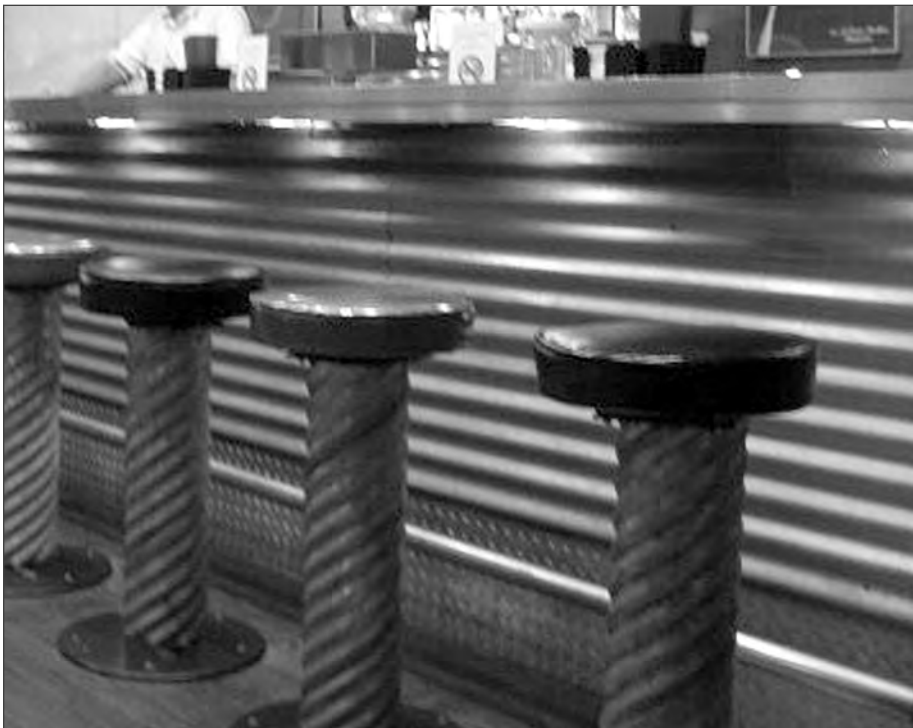
■ CSP and structural plate used in interior design.
