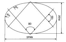
Height-of-Cover Limits for Structural Plate Horizontal Elliptical Pipe E80 Live Load • 6 x 2 in. Corrugation
