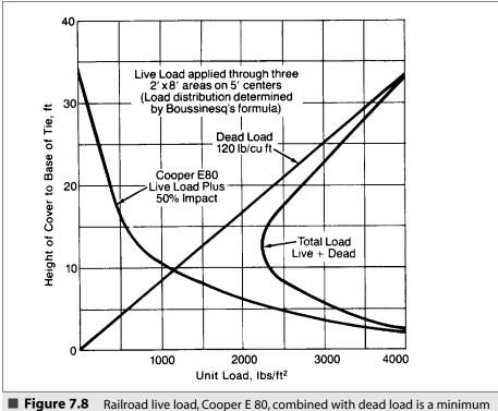
**Figure 7.8** Railroad live load, Cooper E 80, combined with dead load is a minimum at about 12 ft. Live load is applied through three 2 ft x 8 ft areas on 5 ft centers.
