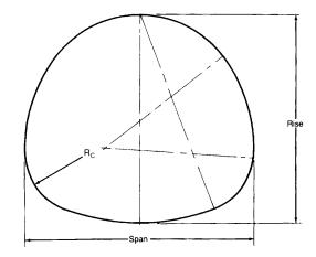
Height-of-Cover Limits for Structural Plate Underpass H20 or H25 Live Load • 6 x 2 in. Corrugation
