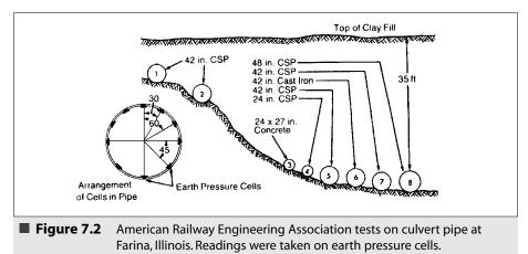
Railroad (1923) demonstrated early on that corrugated steel pipe carries only a portion of the expected load. These tests indicated that the pipe typically carried about 60 percent of the load and the backfill envelope carried the other 40 percent.
