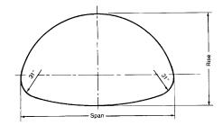
Height-of-Cover Limits for Structural Plate Pipe Arch  $\cdot$  31 in. R<sub>C</sub> Corner Radius H20 or H25 Live Load  $\cdot$  6 x 2 in. Corrugation
