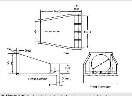
**Figure 7.25** Treatment of outlet end of large corrugated steel structures.
