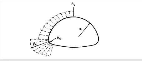
**Figure 7.11** The pressure on a pipe arch varies with location and radius, being greatest at the corners.
