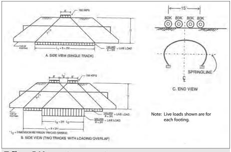
**Figure 7.16** Details for calculating footing reactions with E80 railroad loads.
