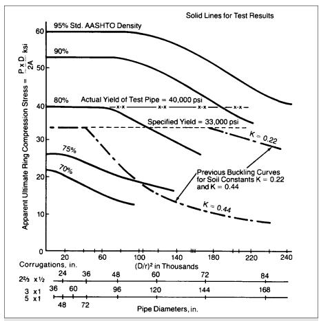
**Figure 7.4** Results of Utah loading tests on corrugated steel pipe, showing apparent ultimate ring compression stress as a function of diameter and corrugations of various values of soil density determined by AASHTO standards.
