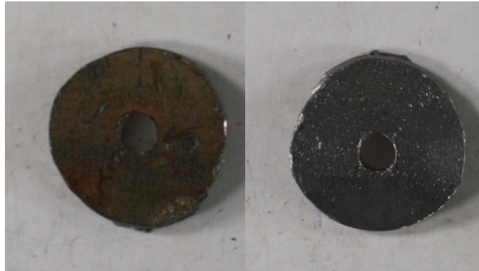
Fairplay, CO “as-received” Fairplay, CO “post-blasting” Figure 1. Representative Sample Cleaning
