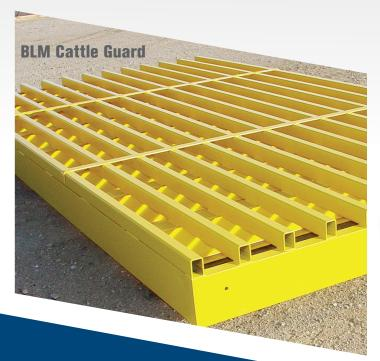
**Bureau of Land Management** cattle guards are made using 3"x2" square high-strength steel and are fabricated to BLM specifications. These cattle guards are typically painted using Federal Safety Yellow but can be painted per project specifications as they are made to order. Holes are provided for multiple cattle guard assembly.
